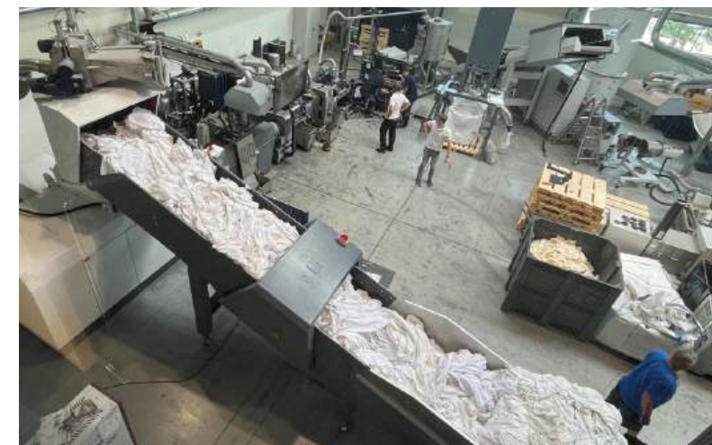
Fig. 2 Detection of metal from the uniforms before the polyester is melted into pellets
