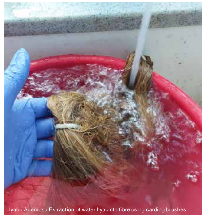
Iyabo Ademosu Extraction of water hyacinth fibre using carding brushes
