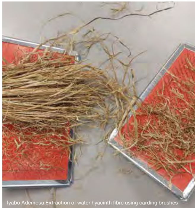
Iyabo Ademosu Extraction of water hyacinth fibre using carding brushes
